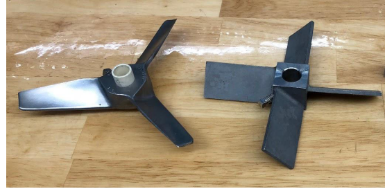
Figure 1: A310 (left) and A200 (right) impellers
