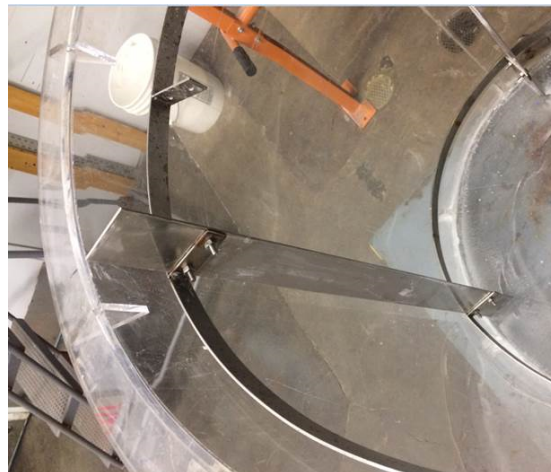
Figure 4: New baffle design, photo from SPX Lightning
