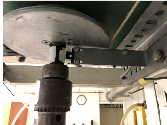
Figure 2: Tachometer in tank setup
